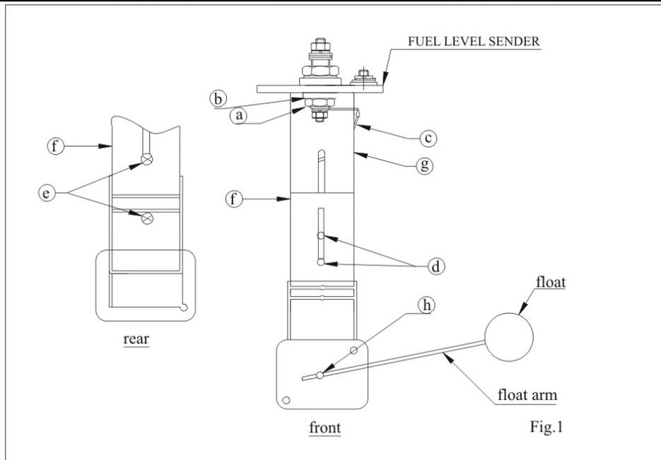
III. For tank depths of 16" to 21" no disassembly of the sender bracket is necessary.
